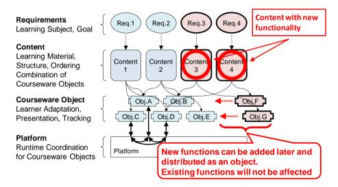
Figure 2. Configuration of the proposed learner-adaptive system
