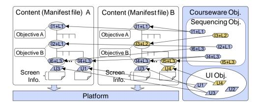
Figure 3. Configuration of the proposed system treating hierarchical content
